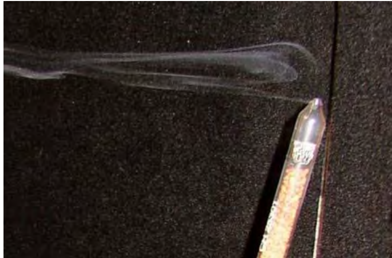
Figure 13 Visible smoke plume emission from a smoke pencil
