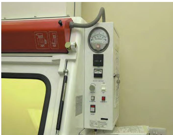
Figure 8 Alarms/indicators on safety cabinet
