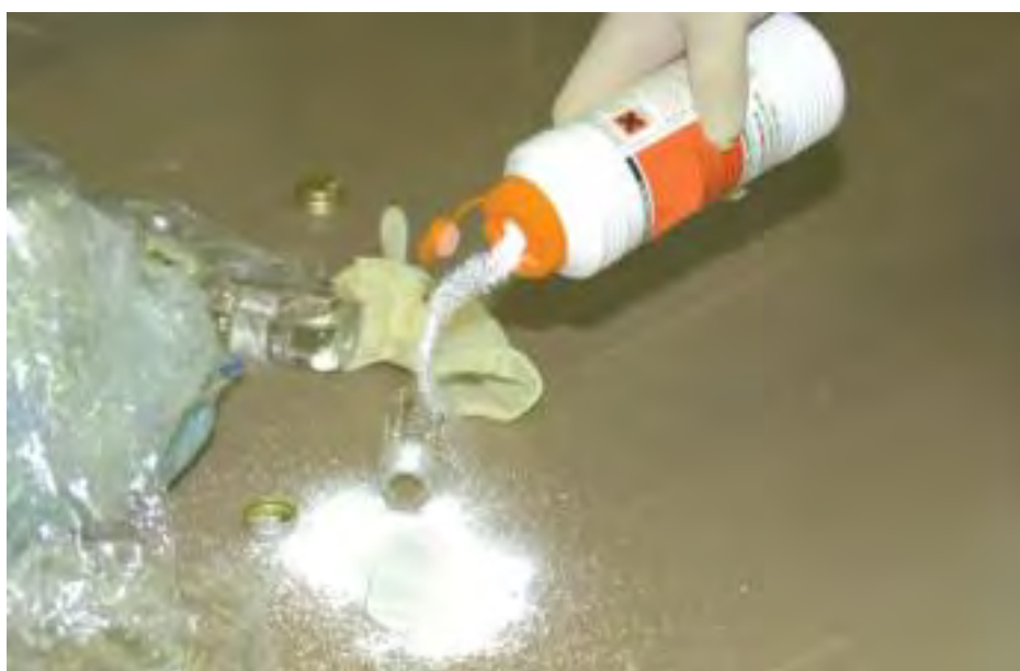
Figure 16 Clearing up a small liquid spill
